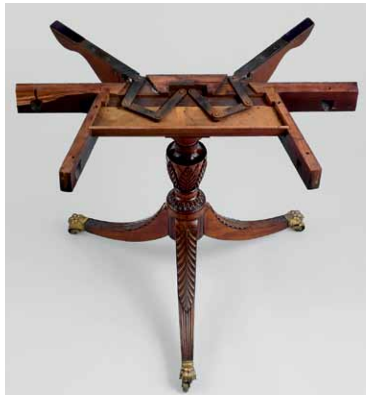
Figure 76. Detail of the trick-leg mechanism on a New York card table, ca. 1810. The Metropolitan Museum of Art, The Sylmaris Collection, Gift of George Coe Graves, 1930 30.120.16
